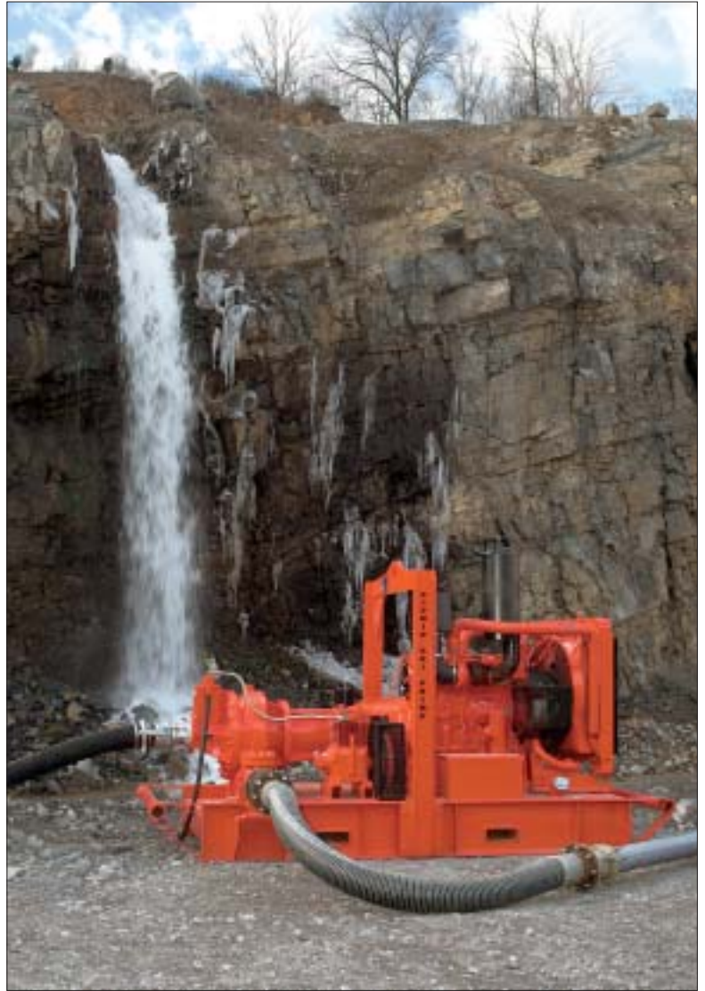
Godwin HL130M single stage Dri-Prime pump achieves heads to 185 metres
